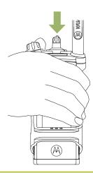
3 To remove the radio from the carry holder, place the tip of your fingers on the ledge of the carry holder.
