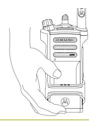
**4** Push at the bottom of the radio until the radio is released from it.
