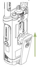
2 Use a flat-bladed object to press the belt clip tab away from the radio. Then, slide the clip downward and away from the radio to remove the clip.
