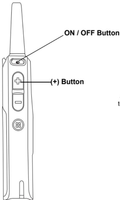
Power UP using the ON / OFF button while pressing the PTT and (+) buttons simultaneously to enter Advanced Configuration Mode
