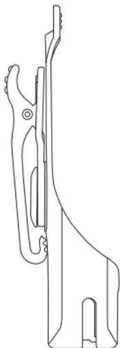
1. Insert the radio into the base of the holster at an angle. Press the radio against the back of the holster until the hooks on the holster are inserted in the top recesses of the battery.
