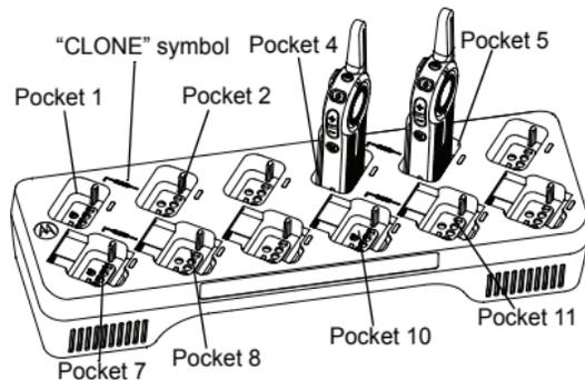
To clone radios using the MUC, there must be at least two radios:
