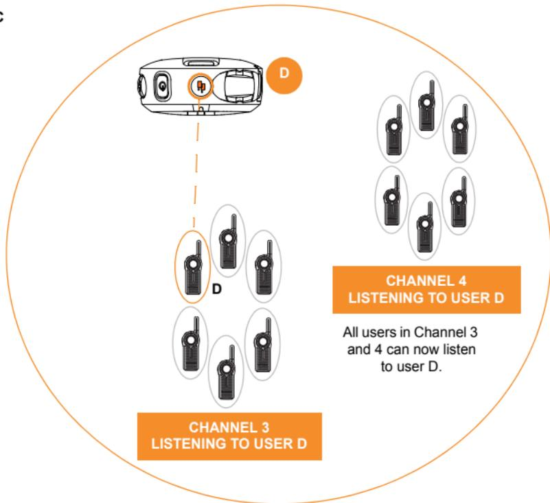
4. All radios Top Buttons in Channel 3 and 4 are **solid orange** indicating that Call All Available is in progress.
