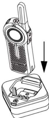
The DLR Series radio comes with a Standard Power Supply and DLR SUC tray.
