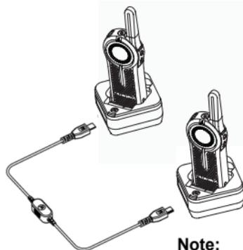
**Note:** Uses Cloning Cable P/N# HKKN4028\_
