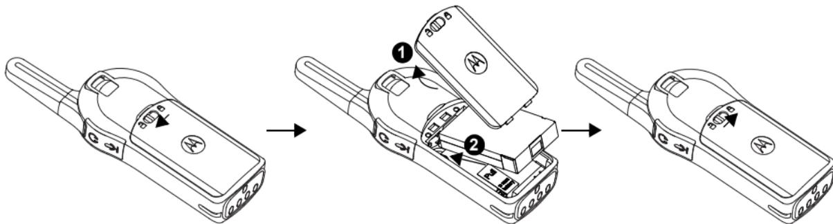
1. Slide the latch at the top of the battery door to the unlock position
