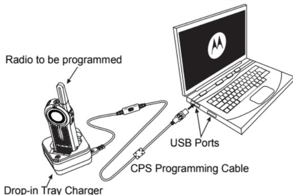
**Figure 1:** Setting up the radio to the CPS
