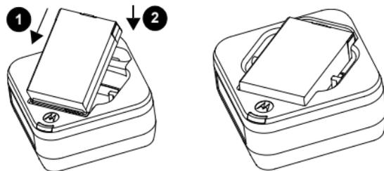
To charge a battery, insert the battery into the charger's pocket by:
