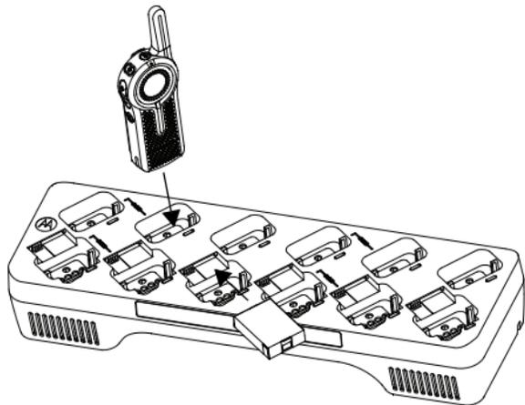
The DLR 12-Pocket Multi-Unit Charger (MUC) allows drop-in charging of up to 12 radios or up to 6 radios and 6 stand-alone batteries. Batteries can be charged with the radios or removed and placed in the MUC separately. Each of the 12 charging pockets can hold a
