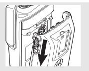
2 Pull the top of the battery away from the radio.
